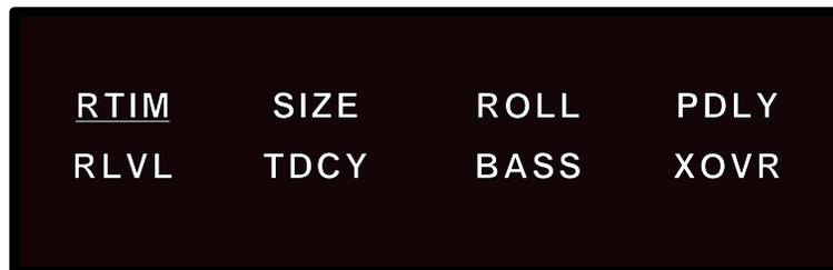
The buttons directly above and below each display entry will select that parameter. Once selected, parameters can be adjusted over their entire range with the Soft knob. The parameter and its current value will appear on the display as long as the Soft knob is being adjusted. In the example above, "RTIM" has been selected — turning the Soft knob will alter the parameter value, and cause the display to show:
