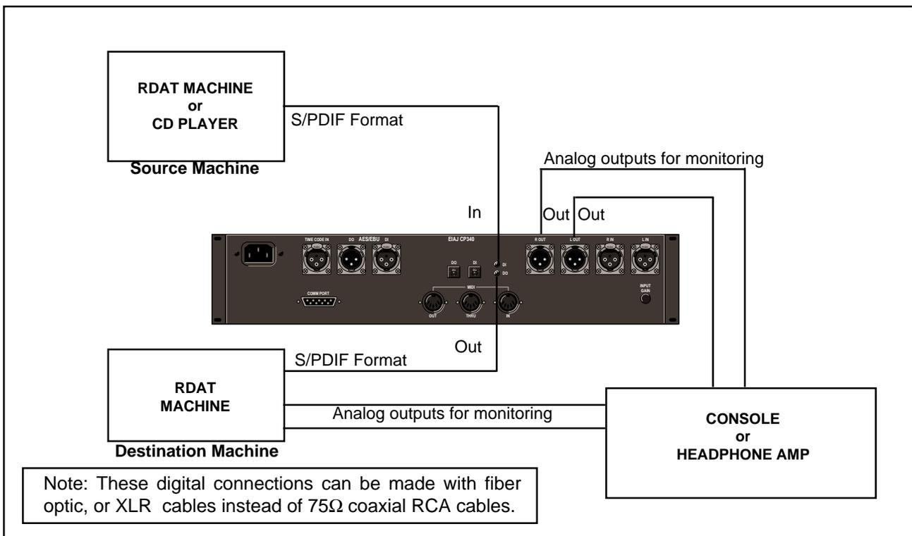
Note: These digital connections can be made with fiber optic, or XLR cables instead of 75Ω coaxial RCA cables.
