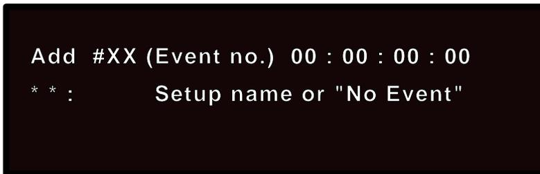
The ADD function is used in two different ways. To duplicate an event, press the button directly above the Event number field and use the Soft knob to scroll to the event that you want to copy. When you press STORE, the event will be copied. (The copy will be placed directly after the original on the list.) To edit the event effect, return to the main Time Code menu (by pressing CONTROL), then press the button directly above "EDIT".
