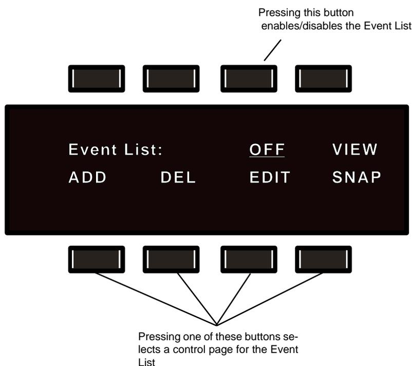
Pressing the second button from the right on the top row allows you to choose to have a Timecode Event list enabled (ON) or disabled (OFF).
