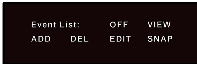
This page allows creation and modification of a list of up to 50 events triggered standard timecode or MIDI timecode. Four main functions are provided: Add, Delete, Edit and Snap. (For more information, see Chapter 6: *Time Code Operation*.)
