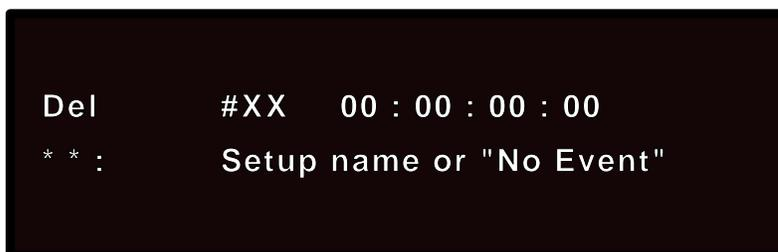
Selecting #XX allows soft knob selection from among the Event List entry numbers (1-50). The time code associated with the event number is displayed to the right. Press the key directly above "Del" to delete any event number from the list. Note that if an entry number is deleted from the list, all subsequent entries will move up on the list.
