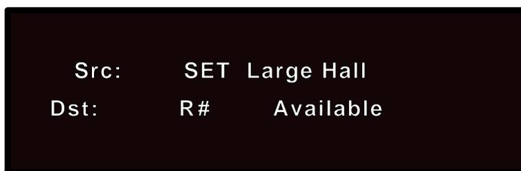
The top line of the display shows the source (Src) — the currently selected setup name. The bottom line shows the destination (Dst) — the register number into which the the setup will be copied. Use the Soft knob to select the register number you want, then press STORE again. The display will return to the last Setup Edit page.
