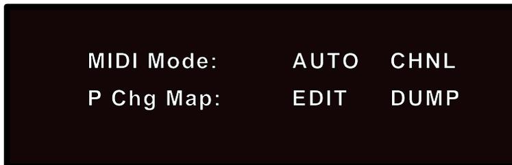
On the upper line, selecting "AUTO" activates output automation on the 300. The choices are OFF, SysEx, Non-registered parameters, and Program Change Only. When the AUTO Mode is set to "OFF", the 300 will not output MIDI data.
