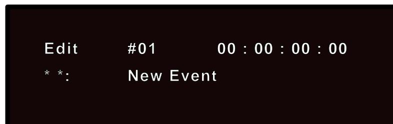
Press the key directly beneath “\*\*\*”. Use the Soft knob to select the automation type. Turn the Soft knob clockwise or counterclockwise to cause the letter S to appear.
