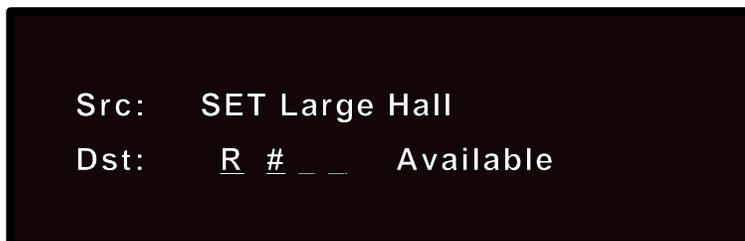
The top line of the display shows the source (Src) — the currently selected setup name. The bottom line shows the destination (Dst) — the register number into which the the setup will be copied. Use the Soft knob to select the register number you want, then press STORE again. The display will return to the last Setup Edit page.
