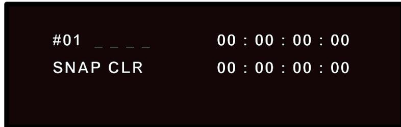
The number displayed in the upper left portion of the display indicates the event number which you are about to snap. Simply press the key directly below "SNAP" wherever you want effect changes to happen. This will assign those time code addresses to the Event List.
