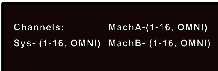
Press either of the left hand buttons in the lower row to select the MIDI Channel for SysEx system and effect changes. Setup patch channel assignments are also set here. Press either of the right hand buttons in the Upper row to select the MIDI Channel for Dynamic MIDI® parameter changes for Machine A. Press either of the righthand buttons in the lower row for Machine B. (All selections may, of course, be set to the same channel.)
