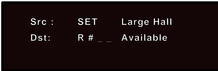
Select "Src" and use the Soft knob to designate a setup number (or the current setup) to be copied; select "Dst" and use the Soft knob to specify the register number where you want this copy stored. When you have made these selections, press STORE.
