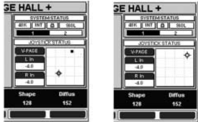
Figure 4-14 — Joystick Status Screen with joystick not locked (left) and locked (right).
