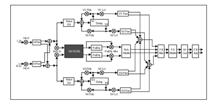
This algorithm emulates a real concert hall. The reverberation is very clean, and designed to remain behind the direct sound — adding ambience, but leaving the source unchanged. This effect has a relatively low initial echo density which builds up gradually over time.
